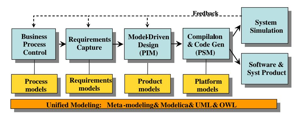
Vision of unified modeling framework for model-driven product development from platform independent models (PIM) to platform specific models (PSM)
