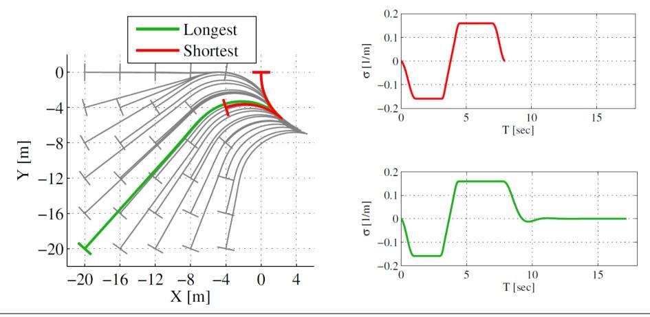
Optimal lifting and Path Profiles for a Wheel Loader Considering Engine and Turbo Limitations.
