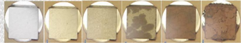
Figure: Carbon steel corrosion in CO<sub>2</sub>, caused by typical CCS impurities
