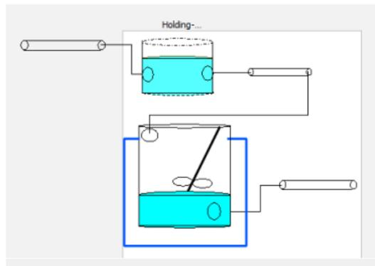
Diagram view of Batch reactor in OpenModelica
