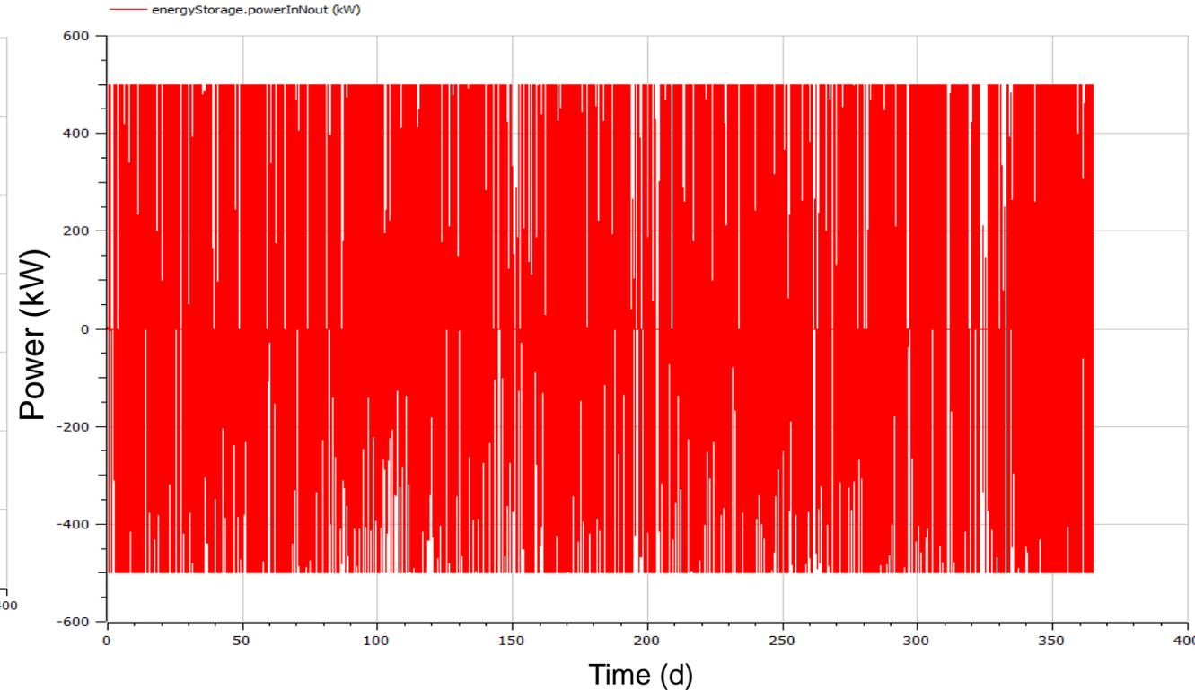
The example plot shows the energy storage Power profile with 500kW Power limit
