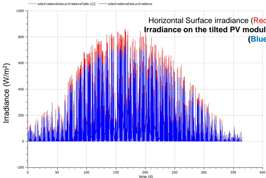
The plot shows the module irradiance for an PV panel with tilt angle = 30deg.
