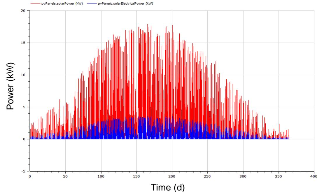
The example plot shows the solar power and the corresponding electrical power generated for  $n=12$  panels of 2m<sup>2</sup> surface area with an efficiency of 20%.
