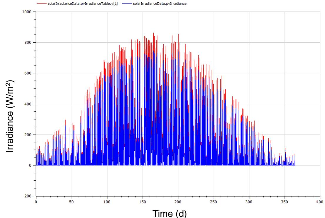
The example plot shows the module irradiance for an PV panel with tilt angle = 30deg.
