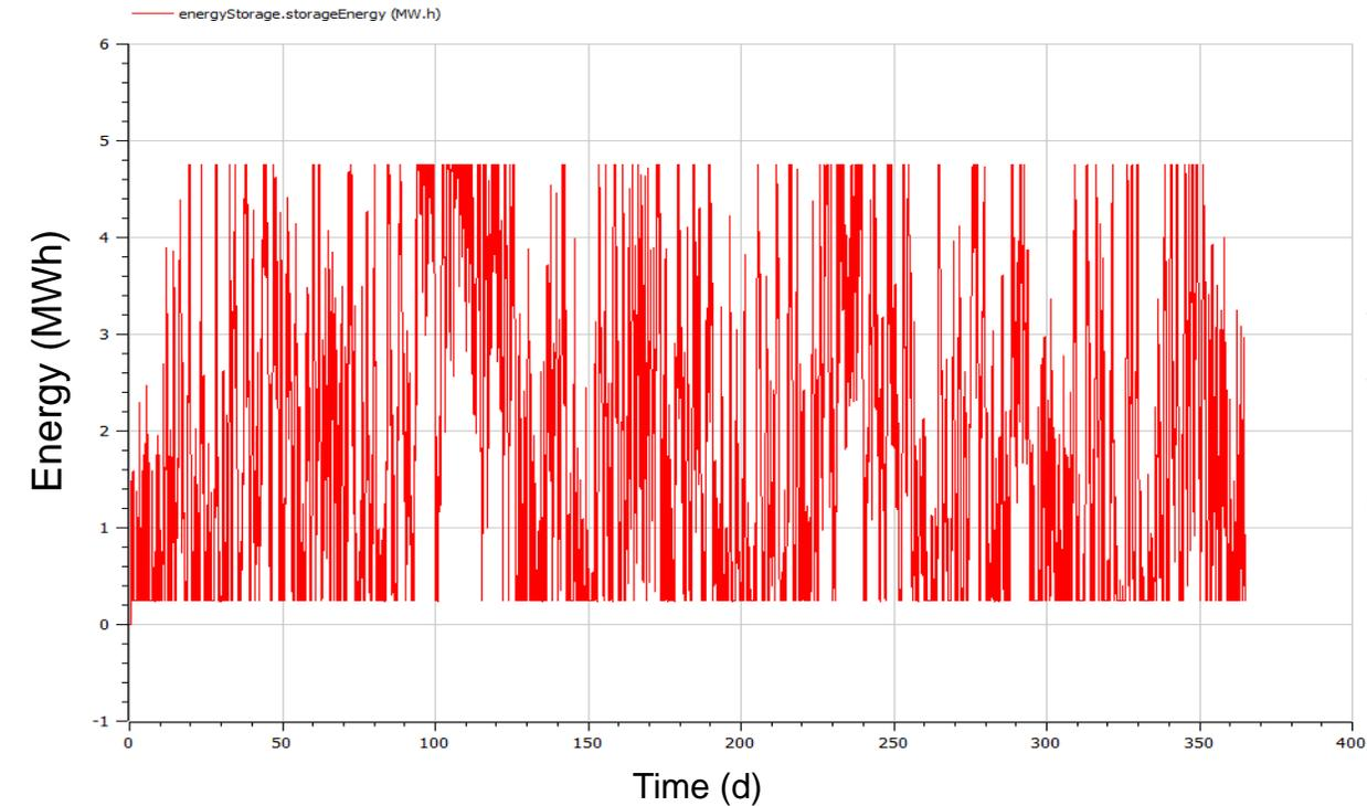
The example plot shows the energy storage energy profile with 5MWh max capacity
