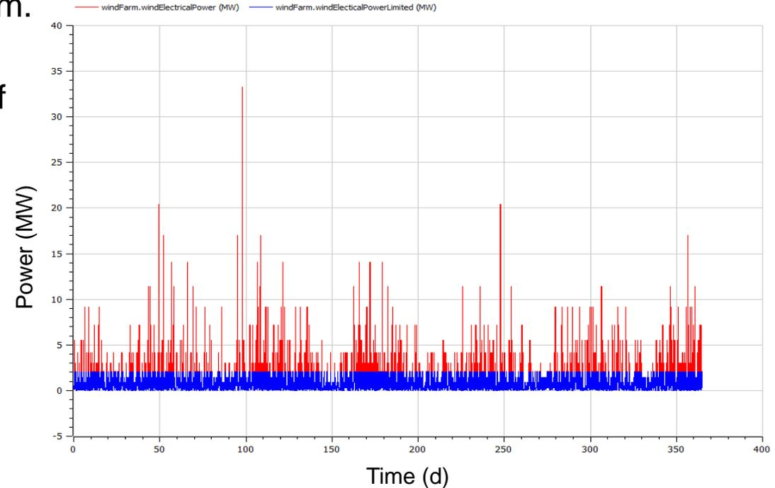
The example plot shows the wind electrical power for  $n=3$  turbines of 30m rotor radius with an efficiency of 80% and rated power of 2MW.
